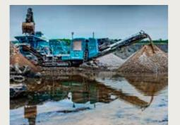
Feeder Crusher Wear resistant feed hopper Vibrating pan and grizzly feeder Twin apron, 4 bar impact crusher Length: 4.87m (15'12") Length: 4.3m (14'1") Feed Opening: 1370mm x 911mm (54" x 36") Width: 2.62m (8'7") Width: 1.26m (4'2") Min. CSS: 75mm (3")\* upper apron Min. CSS: 35mm (1.4") lower apron Capacity: 7m3 (9.2yds3) Grizzly length: 2m (6' 6") Power Unit
