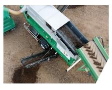
This 55 HP mobile stone separator uses a patented pressure and suction blower system to remove rocks and inert objects from once difficult-to-process output.
