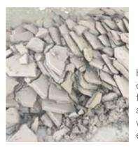
High pressure design leads to faster cycle times and dryer filter cakes which are more easily handled.
