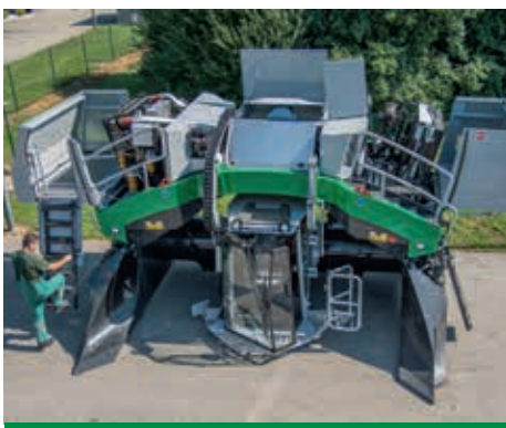
The hydraulically extendable maintenance platforms make for fast and easy maintenance.
