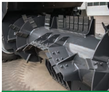
Large diameter turning drum engineered specifically to create the perfect windrow shape.
