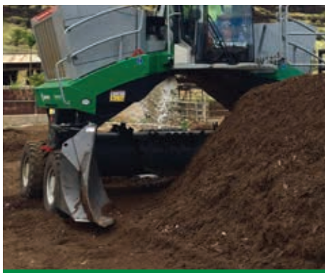
Infuse water into the center of the windrow while turning.
