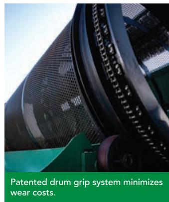
Patented drum grip system minimizes wear costs.
