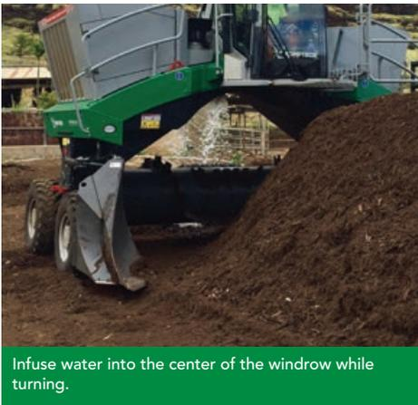
Infuse water into the center of the windrow while turning.
