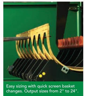
Easy sizing with quick screen basket changes. Output sizes from 2" to 24" .
