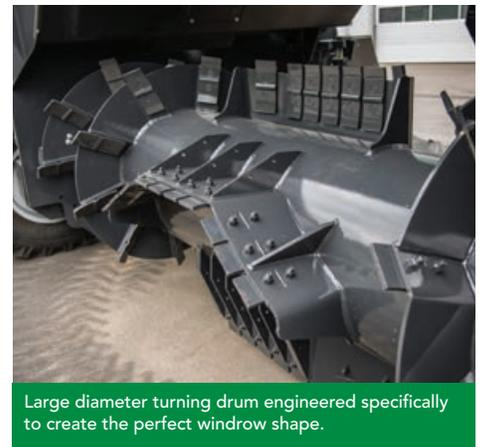
Large diameter turning drum engineered specifically to create the perfect windrow shape.
