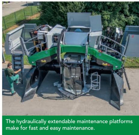
The hydraulically extendable maintenance platforms make for fast and easy maintenance.
