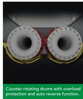
Counter rotating drums with overload protection and auto reverse function.
