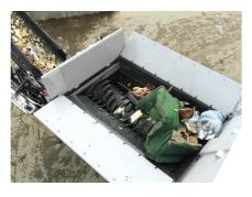
The heavy-duty CAT® engine, high-torque drive, and robust spiral teeth cut, tear, and evenly shred tough waste into variable output sizes.
